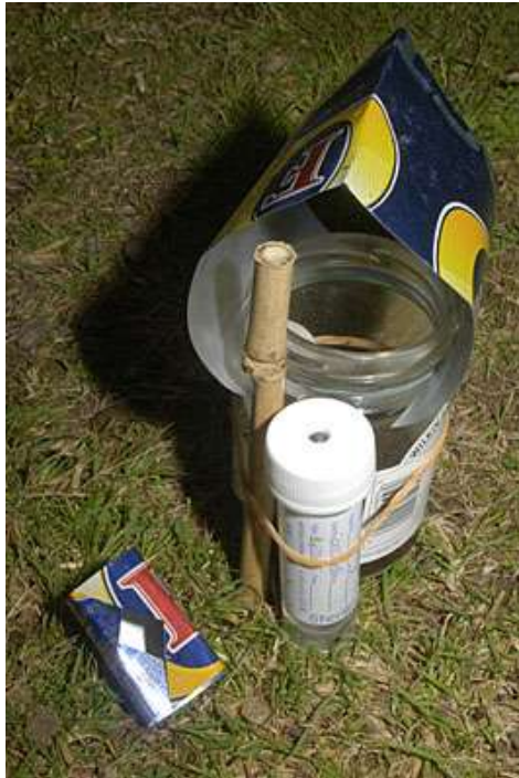
Fig 2: Odour bait containers - acetone in front and cow urine behind. The acetone rain-cover has been removed to reveal its dispensing aperture.
